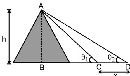
This method is useful in cases when it becomes impossible to measure the distance between the object and the observation point.
