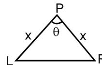
$$\theta = \frac{LR}{x} = \frac{b}{x} \quad (\text{assuming distance } LR \text{ as a circular arc of radius } x)$$
